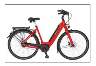
All the Pedelecs are equipped with Bosch mid-drive motors that come with fully integrated 500 watt Bosch rechargeable batteries. The innovative way of construction allows the batteries to become almost invisible. That way, cyclists gain the advantage of a well-balanced bike that is easily operated. It is perfect support and a high level of comfort even on long tours.
