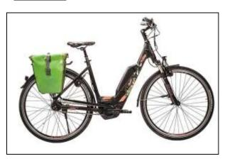
Step through frame, Bosch Performance Line Motor, 8 gear, range performance: approx. 200 km (using middle/constant speed)
