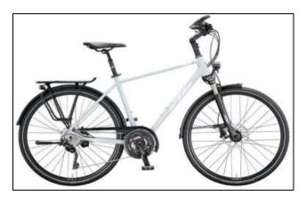
Aluminum frame with bottle holder, with shock absorbing forks, Shimano Deore XT 10x3 gears and Shimano oil disk XT breaks, size S-XL
