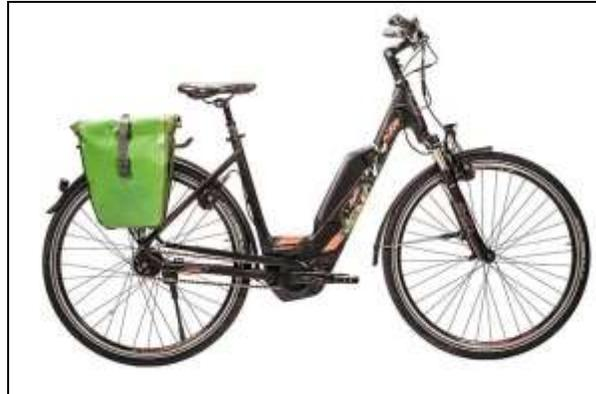
Step through frame, Bosch Performance Line Motor, 8 gear, range performance: approx. 200 km (using middle/constant speed)
