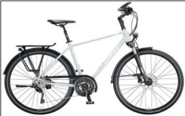
Aluminum frame with bottle holder, with shock absorbing forks, Shimano Deore XT 10x3 gears and Shimano oil disk XT breaks, size S-XL
