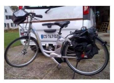
These bikes are supported by an electric motor. The motor is attached to the bottom bracket. The energy supply for the electro engine is retained via a detachable battery, with a possible range of 120 to 180 kilometers. The electro bike is a Pedelec which is an electro bike which assists with electric support only when pedaling.
